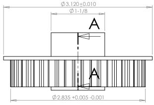
**NOTE: CORED PULLEYS** HAVE 1/16" THICK RIBS, REINFORCEMENT
